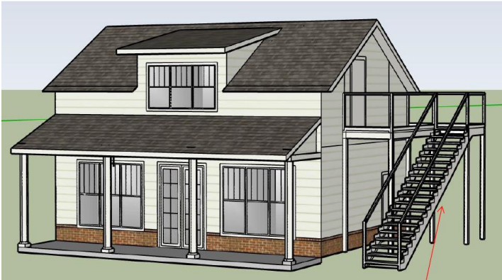
Front view w/single dormer and metal stairs/landing
