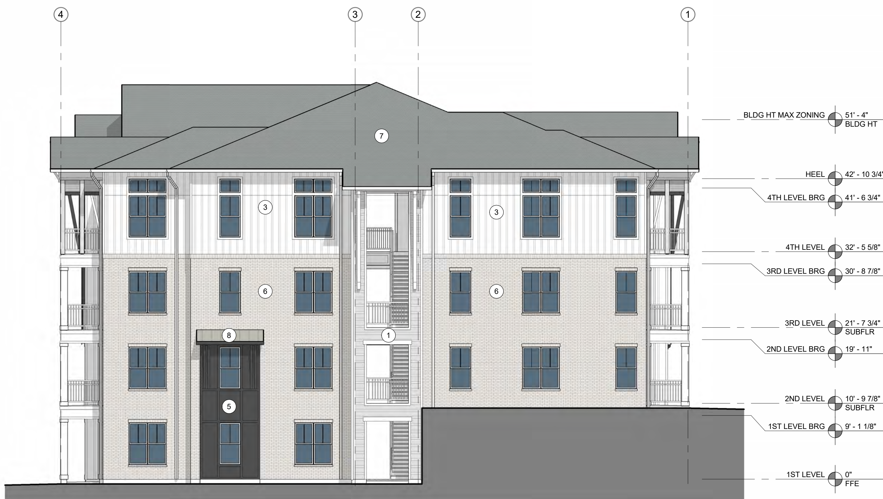
3 EXTERIOR ELEVATION - RIGHT 1/8" = 1'-0"
