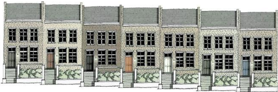
Row facing S. 7 th Street-elevation drops approximately 8 inches per unit due to slope of the land.
