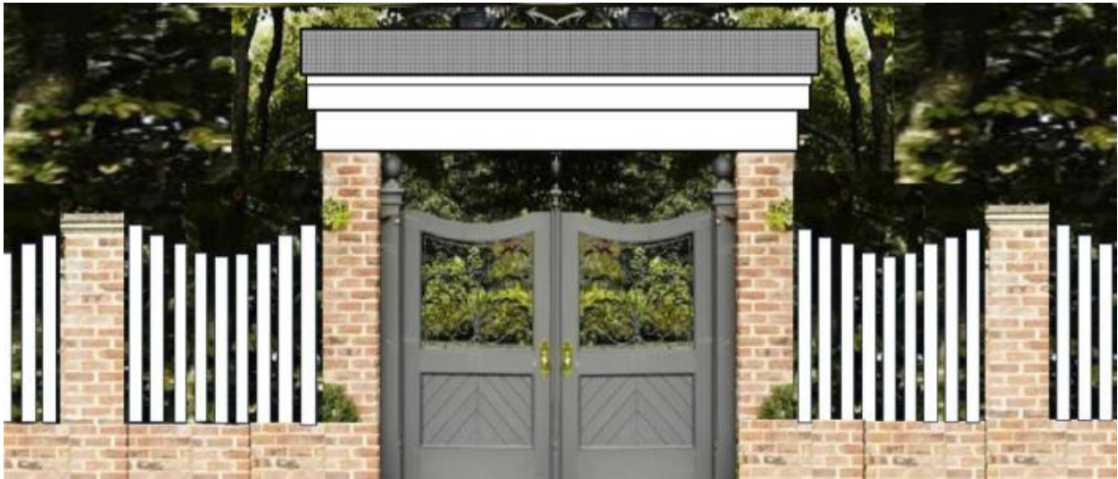
Proposed brick and wood fence with carriage lanterns, capped by architrave, frieze and cornice, and topped with asphalt shingles ~8'-9' in height.
