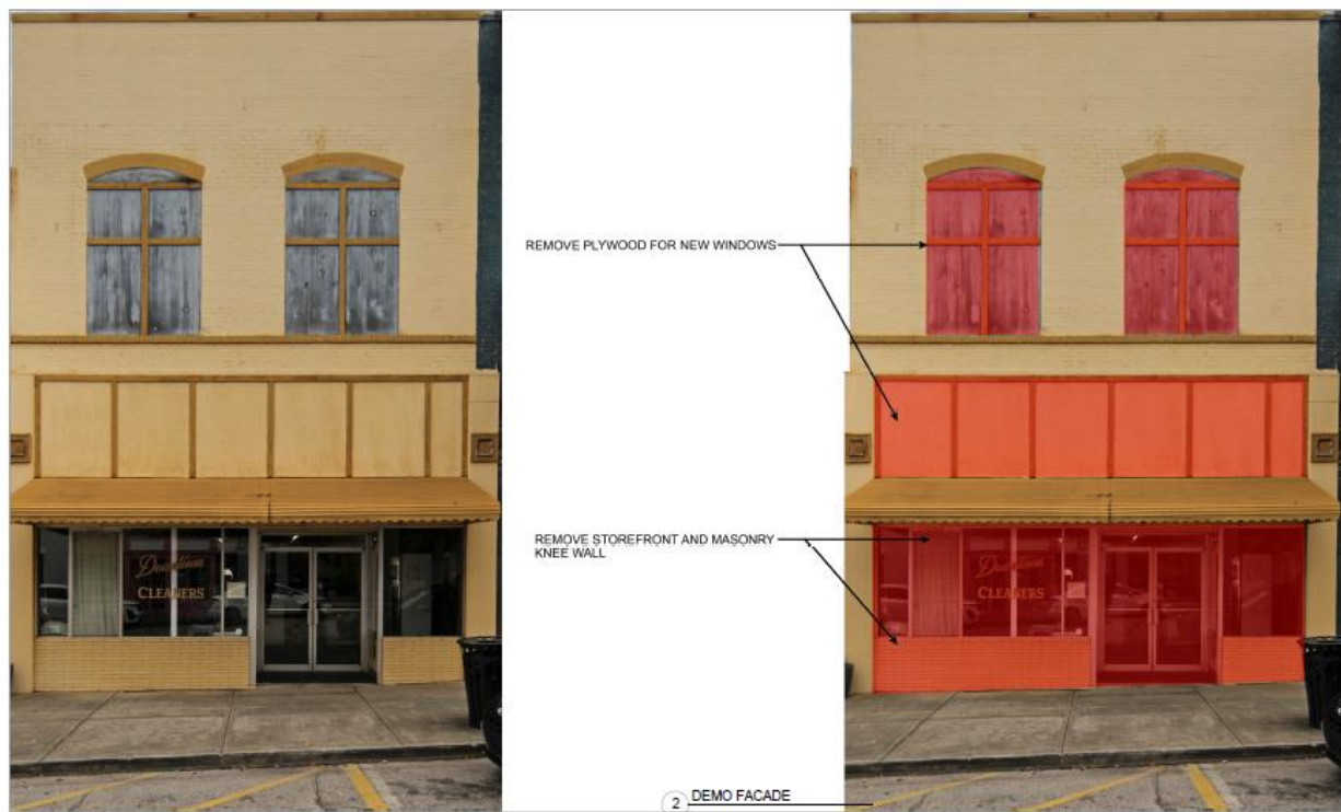
Remove plywood for new windows and Remove storefront and masonry knee wall
