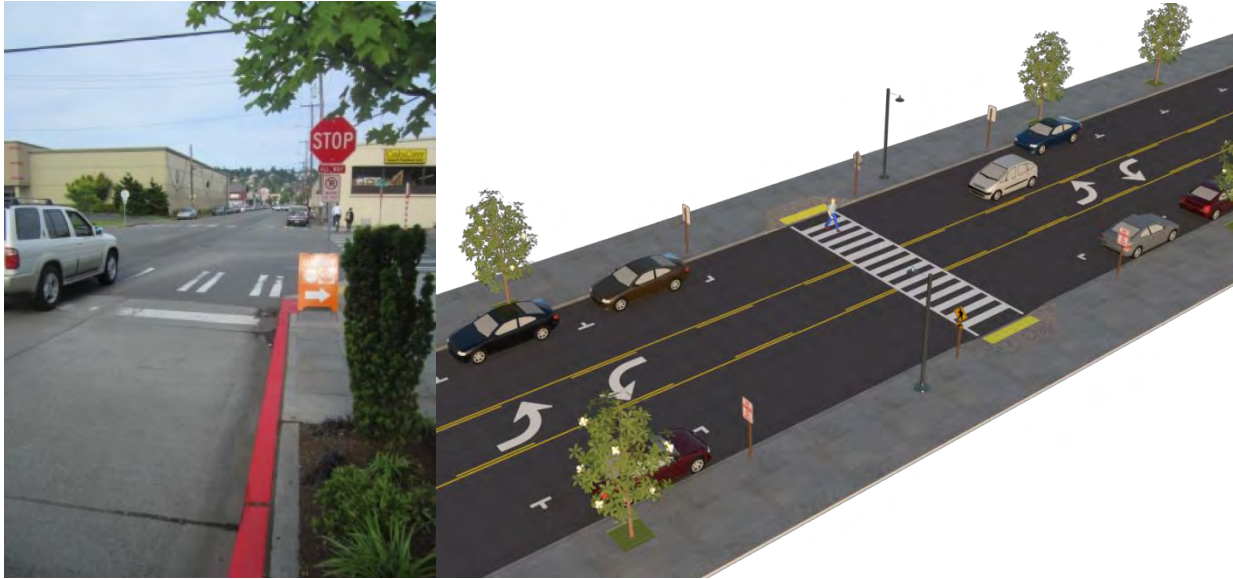
Figure 54: Example of Parking Restrictions at Crossing Locations (Source: PEDSAFE)
