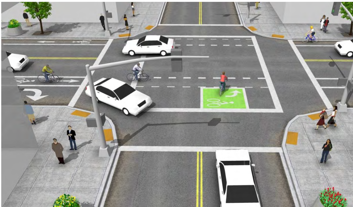
Figure 58: Two-Stage Turn Queue Box Example (Source: NACTO)
