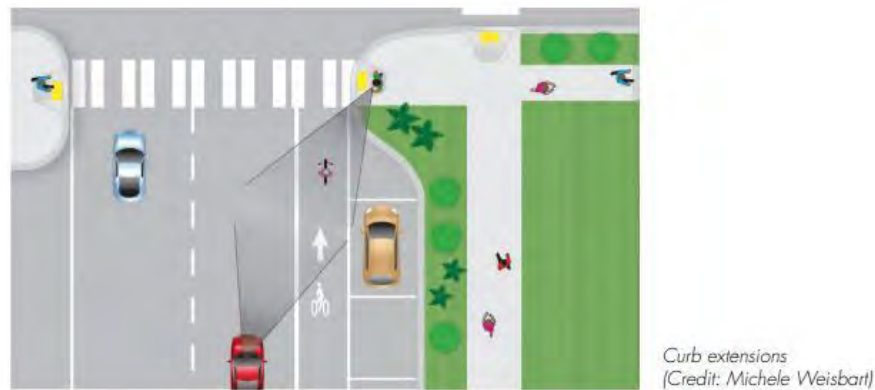
Figure 51: Example of Curb Extensions (Source: PEDSAFE)
