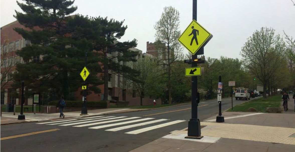
Figure 65: Rectangular Rapid Flashing Beacon Example (Source: PEDSAFE)
