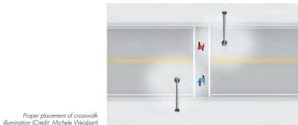
Figure 53: Lighting at a Crosswalk (Source: PEDSAFE)
