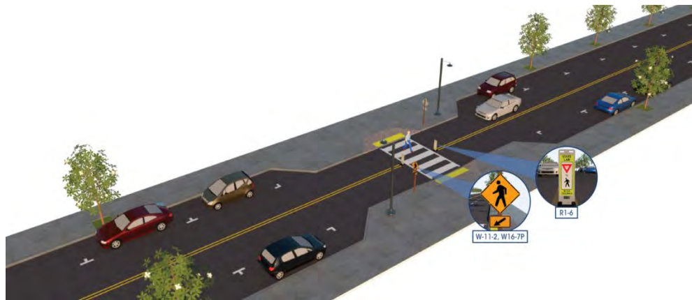
Figure 50: Example of Crosswalk Enhancements (Source: PEDSAFE)
