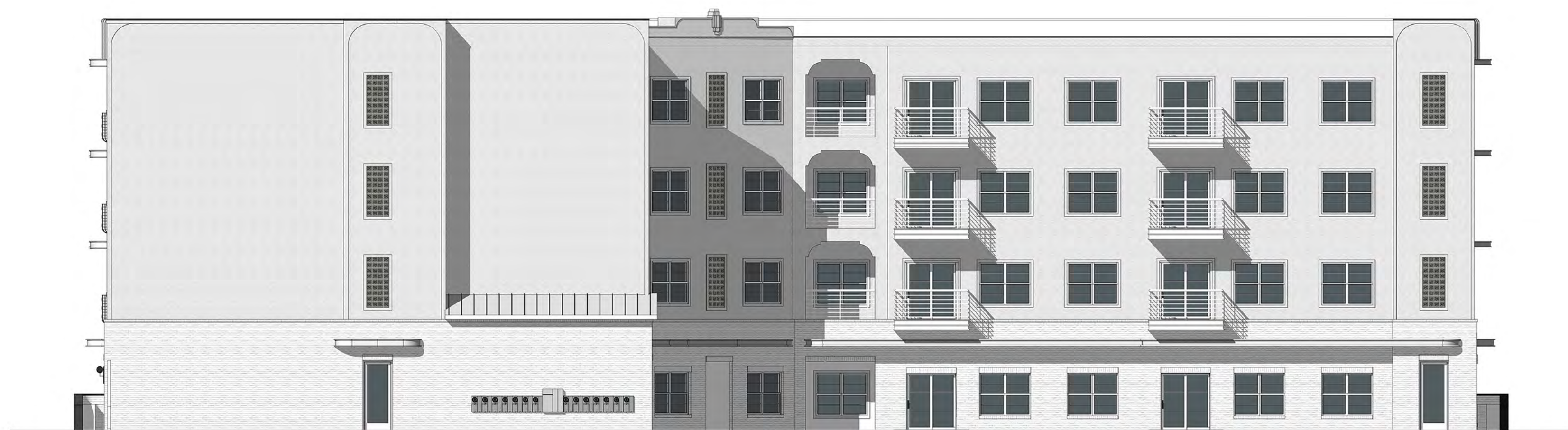
3 SK-1 BUILDING 1 SOUTH ELEVATION SCALE = 3/32" = 1'-0"
