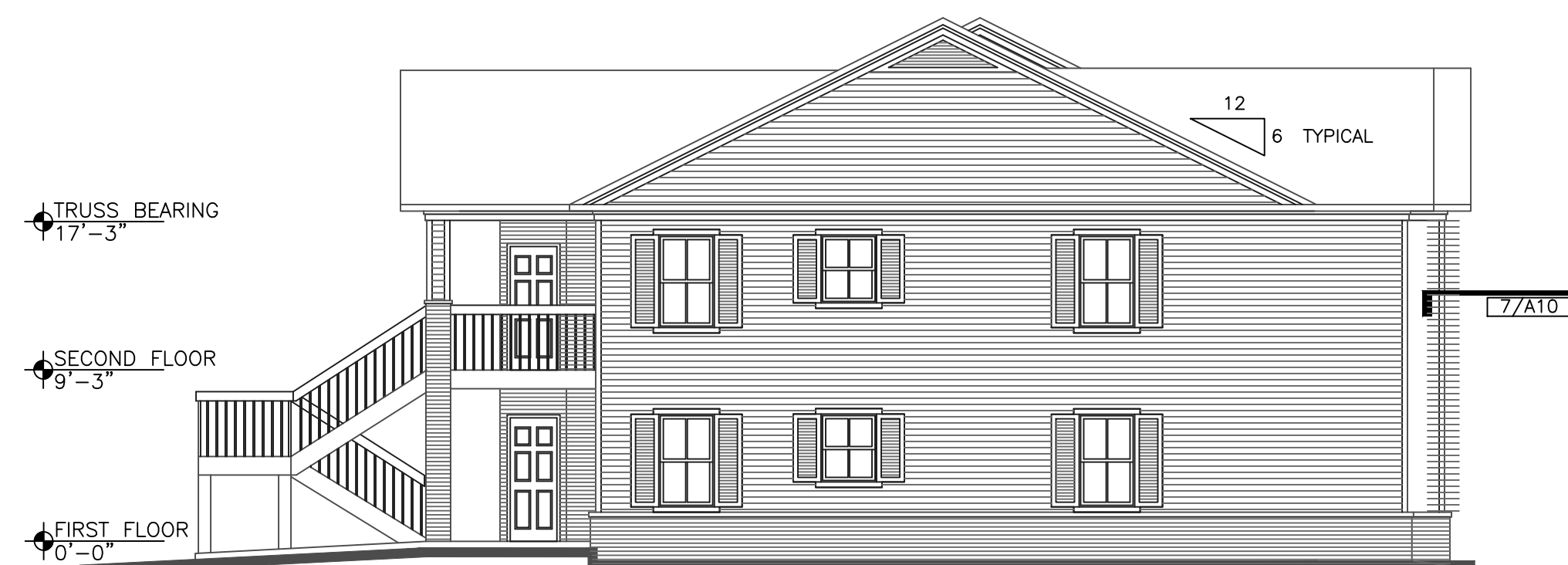
4 SIDE ELEVATION—BUILDING "B2" (SHOWN), TYPE "B1" (SIMILAR OPPOSITE HAND) A07 1/8"=1'-0"
