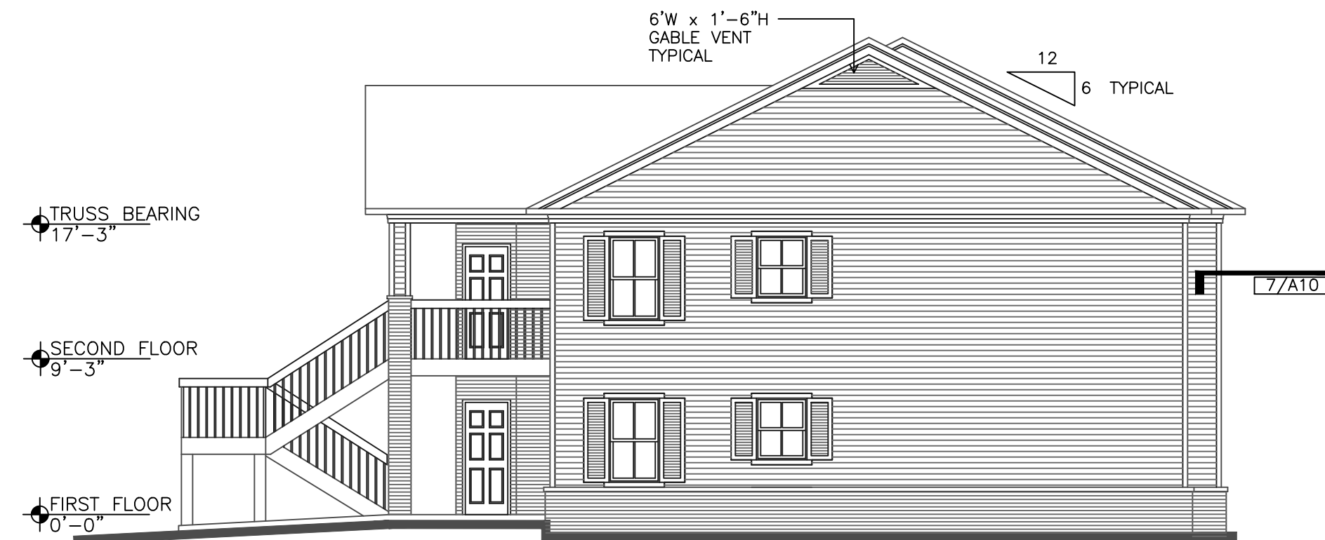
2 SIDE ELEVATION—BUILDING "A2" (SHOWN), TYPE "A1" (SIMILAR OPPOSITE HAND) A07 1/8"=1'-0"
