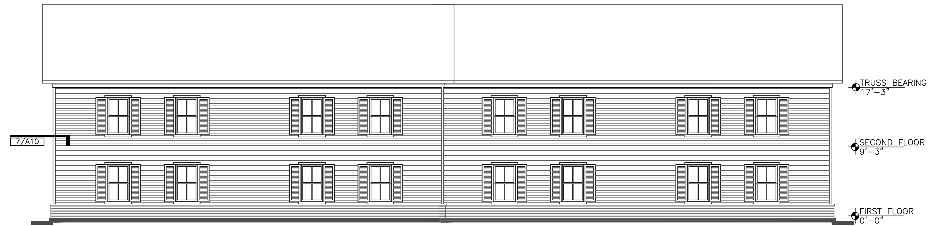
3 REAR ELEVATION BUILDING TYPE "A1" (SHOWN), TYPE "A2" (SIMILAR OPPOSITE HAND) A07 1/8"=1'-0"
