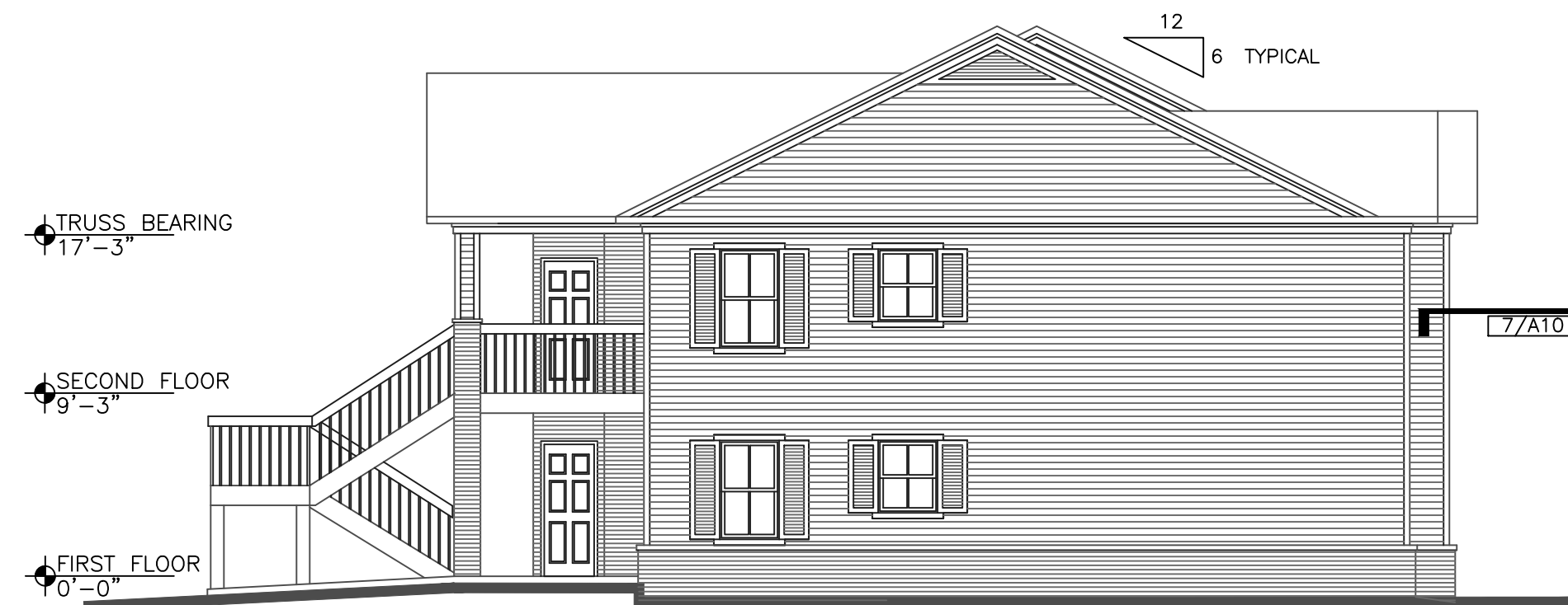
4 SIDE ELEVATION—BUILDING "B2" (SHOWN), TYPE "B1" (SIMILAR OPPOSITE HAND) A07 1/8"=1'-0"
